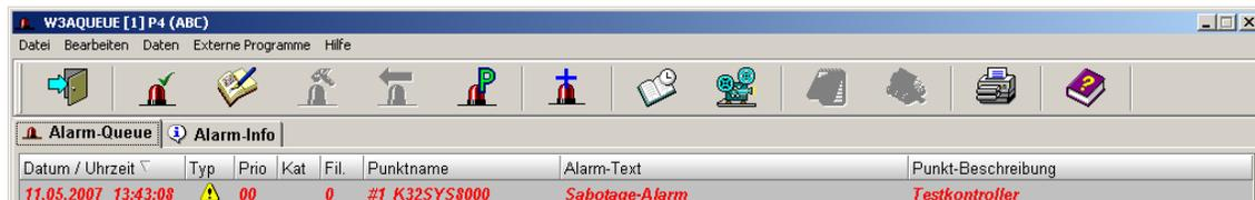
By a double click on the alarm message the actions are displayed which are linked with this alarm – also for displaying a graphic which supports this actions if necessary (e.g. a plan which shows the location where the XMP-K32 is installed).
