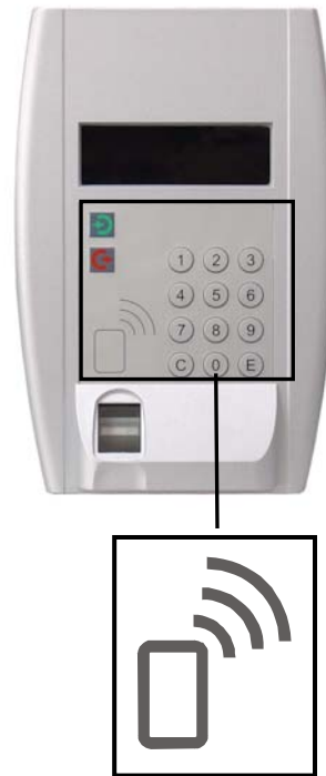
This symbol marks proximity reader head.
