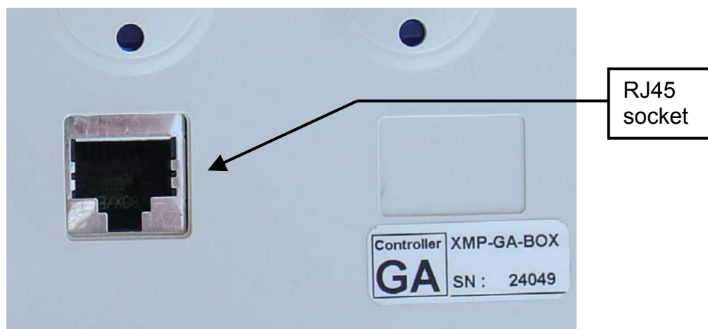
Fig. 3: Connection socket of the XMP-GA BOX
