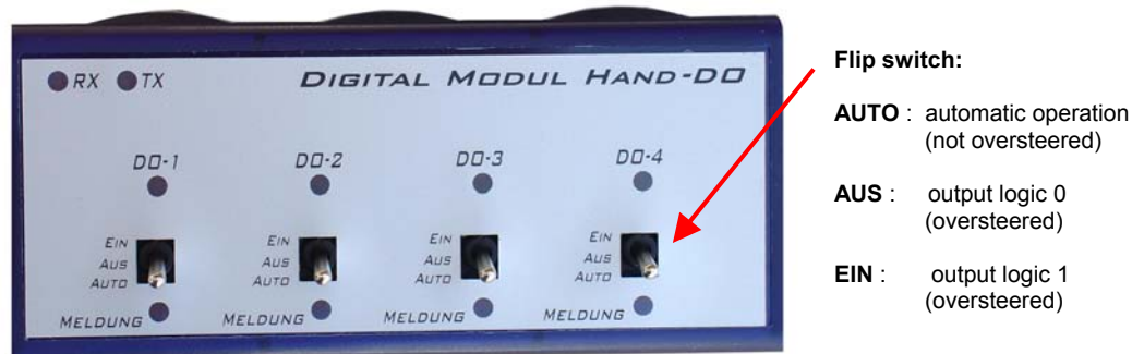
Fig. 22: Module cover of the XMP-GA-HAND-DO module
